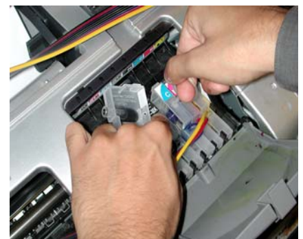
Injector being removed
