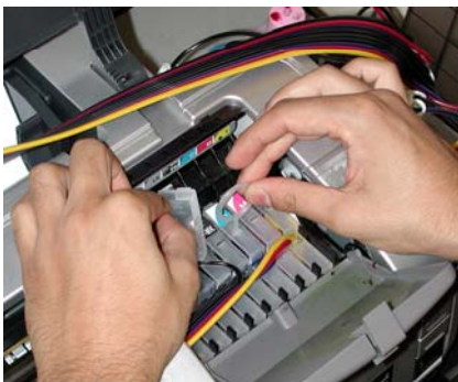
Inserting the tool on the opening slot of the injector
